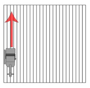
Start from this position. Run the sander along the floor, pulling it up just before you get to the wall. Then, move backwards and lower the drum to sand across the exact same path you have just taken. Don't forget to lift up before you stop!
