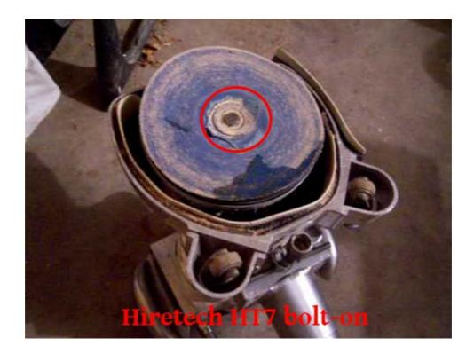
Before you turn on the machine, tip it back on its two wheels so that the disk is not in contact with the floor. Then, turn on the machine before slowly lowering it onto the floor. Again, you don't want to be touching the floor with the disk if you have come to a stop. It isn't quite as important as with the floor sander but you want to keep the machine moving as much as possible to prevent creating dips.
