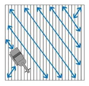
It's important to run over the floor with 36 grit going with the grain if you have previously sanded the floor diagonally in the same way. This is because you want to remove the diagonal scratches and they may not be removed using a higher grit.
